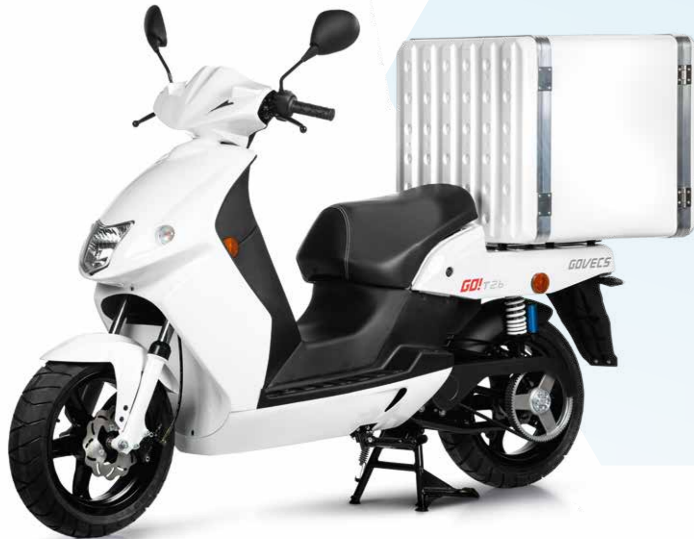
GO! T1.5 Maximum speed: 45 kph Range: 50 – 70 km New 2.1 kWh battery
